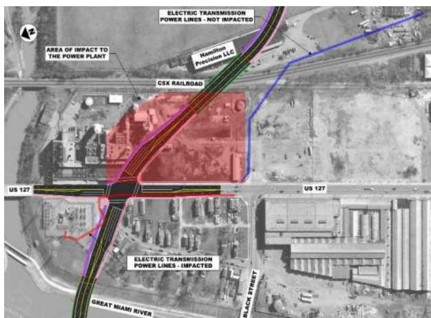
Figure 35: Alternative E1 Impacts to Power Plant and Electric Power Lines
