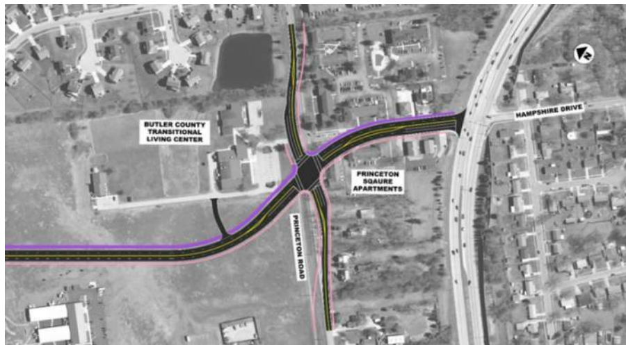
Figure 8: Reconfigured Hampshire Drive/Princeton Road Intersection
