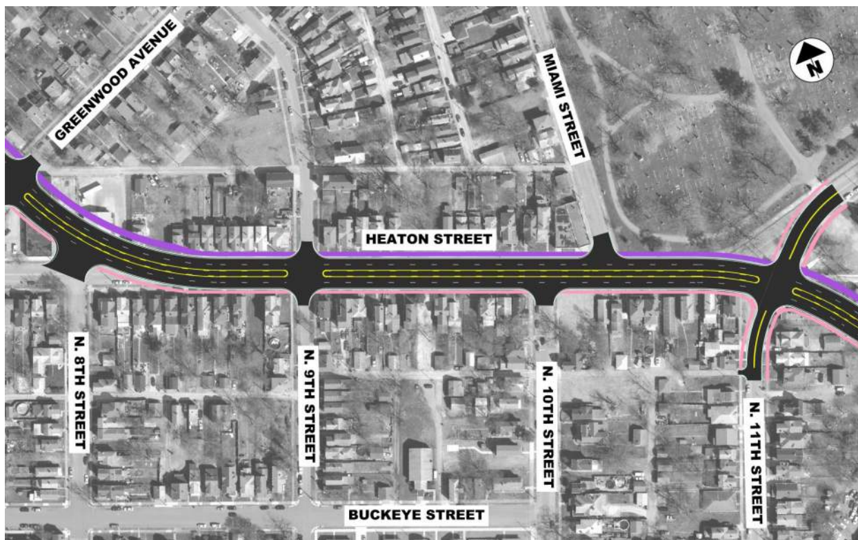
Figure 28: Alternative F1 Reduced Property Impacts Along Heaton Street Due to Reduced Roadway Typical Section and Raised Profile
