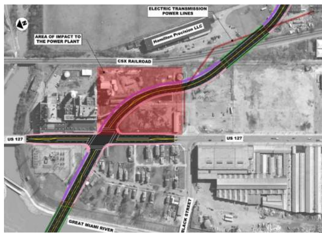
Figure 33: Alternative D Impacts to Electric Transmission Power Lines and Power Plant
