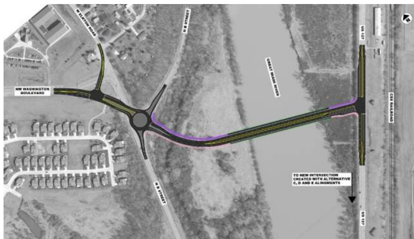
Figure 23: River Crossing and Roundabout at W Elkton Rd and NW Washington Blvd. for Alts. AC, AD, AE, ABE and AF1
