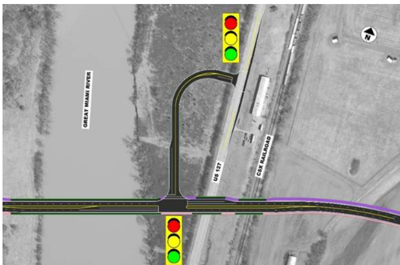
Figure 10: J-Hook Connection at US 127
